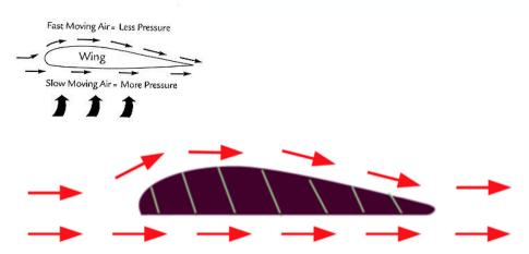
The bottom of the wing is straight. Air moves more *slowly* here. This is an area of **High Pressure**.
